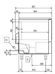
Drain Electrical inlet (power) ΕI Refrigerant Outlet
